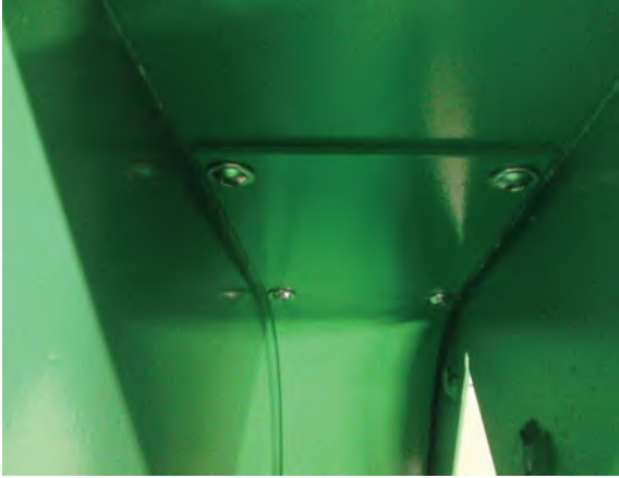
Replaceable housing liner made of HARDOX steel.
