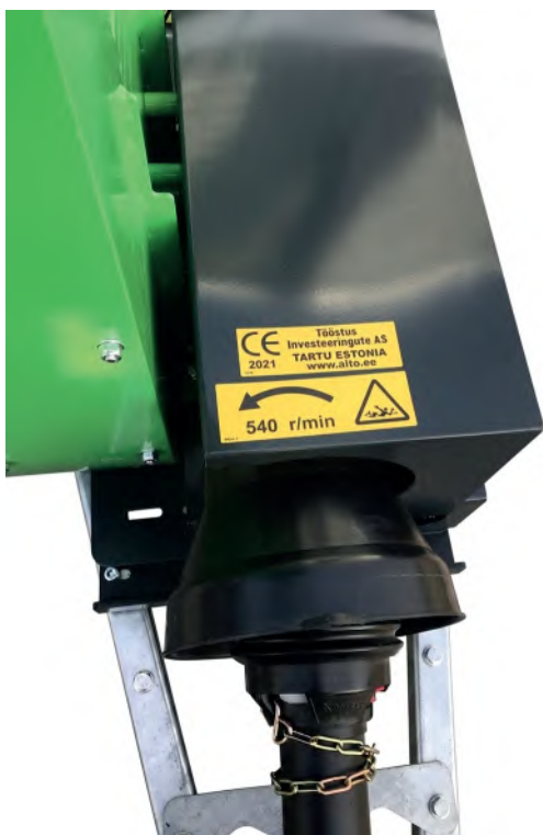
The vacuum's drive consists of a gearbox and a belt drive
