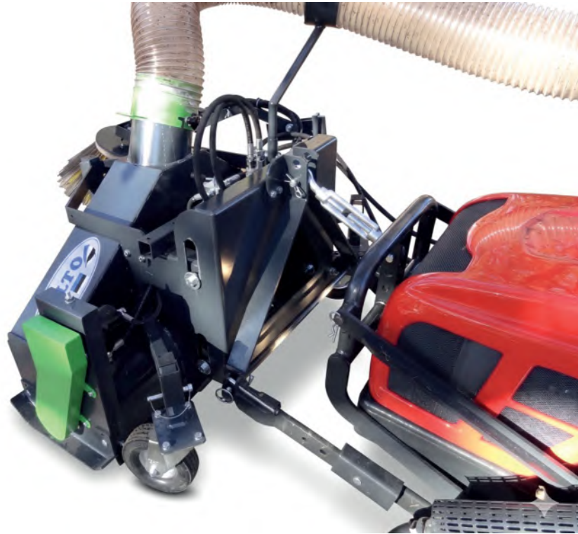
The leaf brush follows the ground; various brush mountings for tractors
