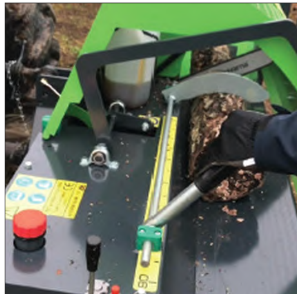
ALTO KSK-50 models have a 13-inch saw bar and a standard saw chain. Max. cutting diameter 30 cm, max. block length 50 cm.
