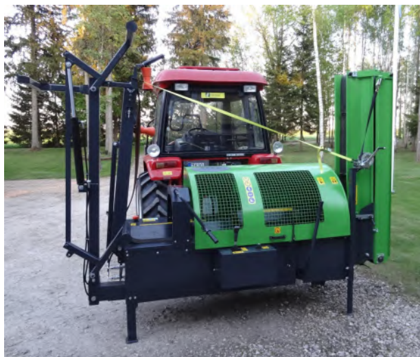
Three-point linkage models can be driven by PTO shaft, electric motor or both.
