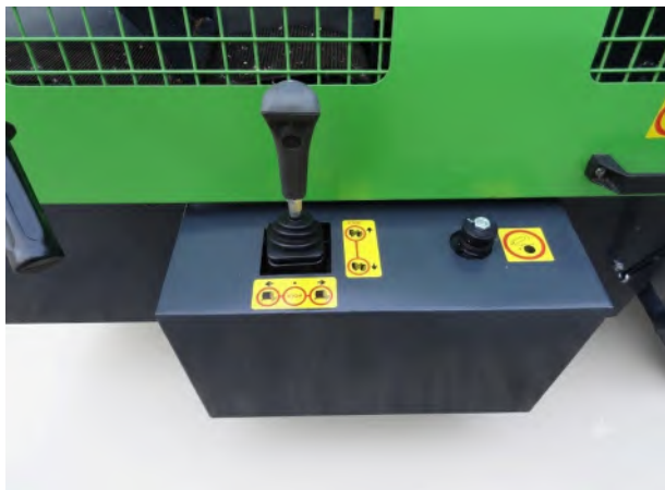
Joystick lever controls the saw bar and the feed conveyor. Saw bar feed speed is set with the hand screw on the right.
